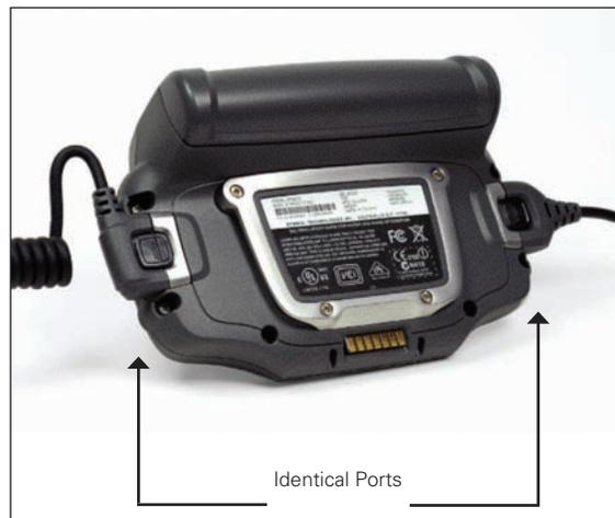
The WT4000 is designed with two identical ports on either side of the product. Each port can be used for either data (scanning) or voice (headset and microphone). This construction allows users to connect peripherals based on mounting preference — left or right arm or belt-mounted.
