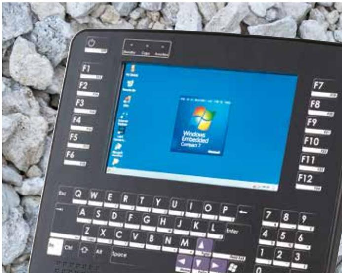
The device is also IP65 rated for full protection against dust, water and oil ingress, can survive 1.5m drops on to concrete, operates in wide temperature extremes (-20°C to +50°C) and has a high impact, stainless-steel chassis.
